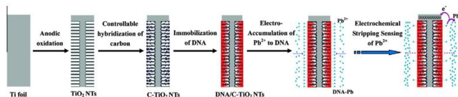
Fig. 7. Schematic illustration for DNA/C-TiO 2 nanotube arrays construction and its Pb ion monitoring [54]
